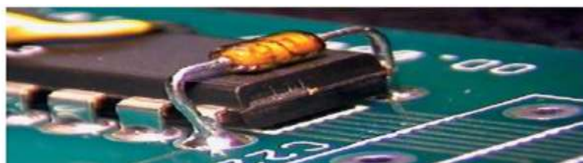
Figure 2 Axial lead component soldered to through hole component leads. Note: Leads of axial component should not be inserted into the plated holes.
