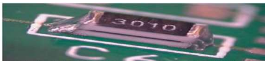
Figure 8 Chip component stacked onto another chip component.
