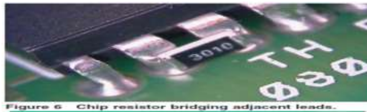
Figure 6 Chip resistor bridging adjacent leads.
